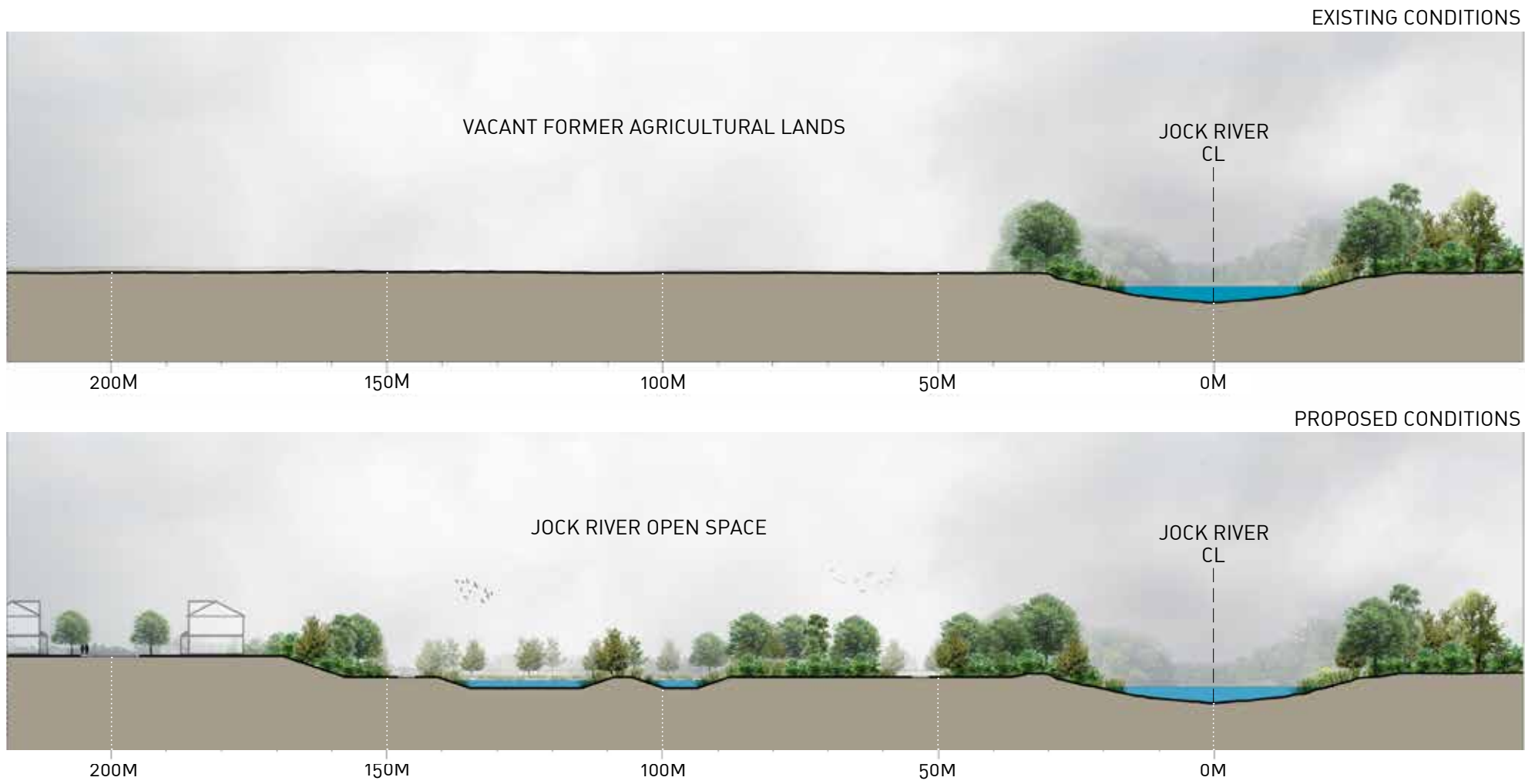
Figure 8 Cross Sections of Existing versus Proposed Conditions
